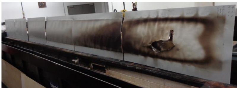
Photo No. 4 Exposed Surface of the Test Specimen (Post-test)
